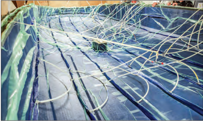
Arkema's recyclable thermoplastic resin Elium was used to infuse the carbon fiber hull ( above ) and deck of a Mini Transat 6.50 ( right ), launched earlier this year in Gironde, France.
